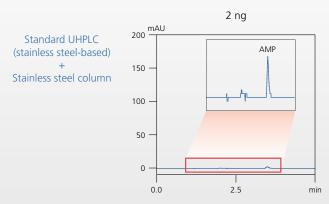
The Nexera XS inert system prevents peak tailing and sensitivity loss by eliminating adsorption of proteins, nucleic acids, and other components to metal surfaces. As a result, reliable and accurate quantitation is possible, even for low-concentration samples or compounds with a strong tendency of metal adsorption, such as oligonucleic acids.
